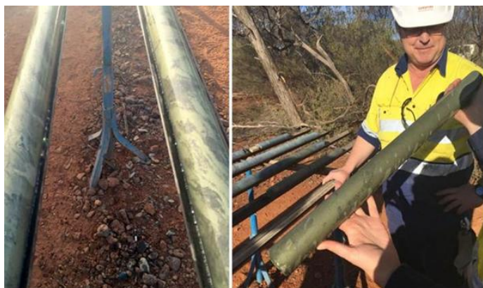
Drilling core from Sandfire's exploration efforts.
